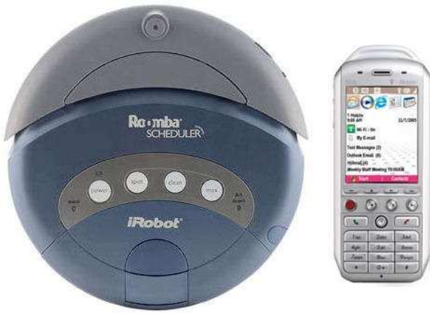
Figure 2: The Roomba Scheduler robot and T-Mobile SDA mobile phone with the Windows Mobile 5 operating system. The port cover for serial communications can be seen in the lower right side of the robot. Figure copyright iRobot, inc., and T-Mobile, inc.
